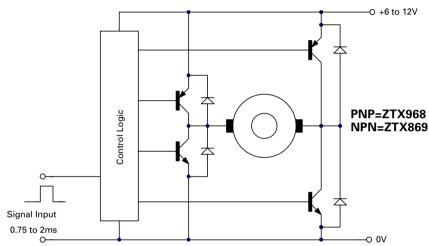
The combined features of low saturation voltage, a 5A continuous current capability, very high gain at high currents, and the compact dimensions of the TO92 style E-Line package, provide an attractive alternative to TO220 devices in this commonly used driver circuit.
