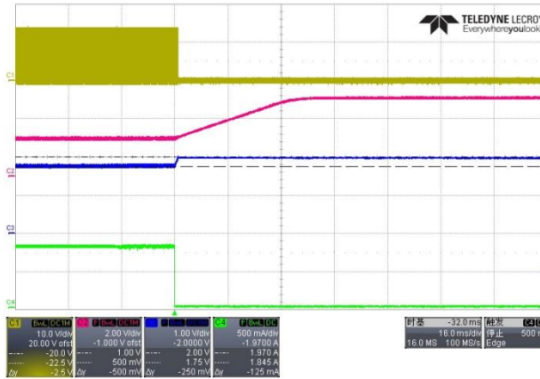
Figure 8: LED Open Protection with 100% Duty
