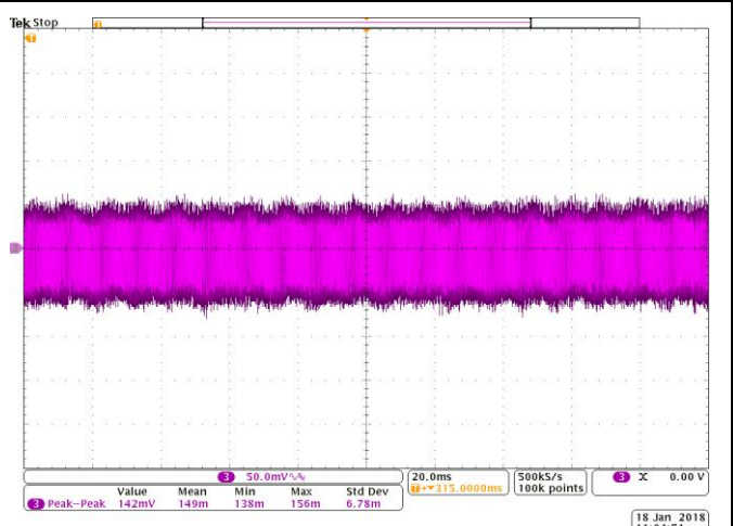
Figure 32: 264Vac/50Hz \Delta V_{P,P}=142mV 5V/3A
